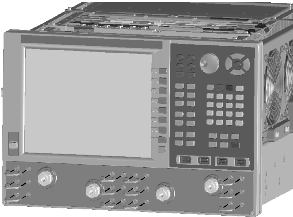
Figure 6 Front Panel Jumper Cables Installation
